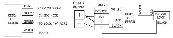
NOTE: Positive input voltage on the white wire must be from same power source that the red and black wires are connected
